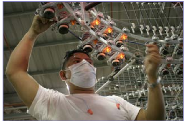
Employee repairing the knitting machine at one of Gildan's supplier facilities.
